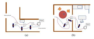
Fig. 7: Two use cases are used in this validation: a) a person who crosses the robot in a corridor; and b) a companion robot moving around an apartment.
