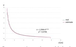
Fig. 5: Power regression used to model the dependence between *sigma* and the distance to the sides, back and front.
