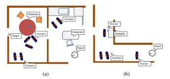
Fig. 1: The robot has to choose the best route and navigate in typical scenarios by using its social rules (a) office environment composed of two rooms; and (b) narrow corridor.
