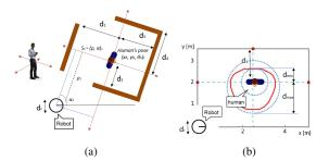
Fig. 3: Description of the method for measuring distances between human and walls. (a) The intersection between the walls and the lines  $S_1$  and  $S_2$  define distances  $d_i$ ; and (b) distances used in the proposed work in order to adapt the personal space to the environment.
