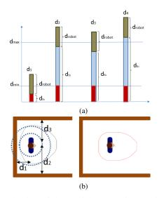
Fig. 4: Evaluation of the spatial context in a typical narrow corridor. (a) Four bars associated to each distance  $d_i$  are drawn. Distance  $d_{s_i}$  identify the need of modifying the comfort zone. (b)  $d_{s_2}$  and  $d_{s_3}$  involve a modification of the personal space in this scenario.
